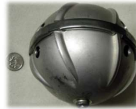
Sarin bomblet showing relative size (USFWS photograph)
